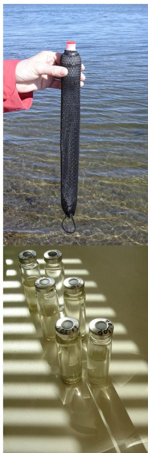
PS VOC, our method for passive sampling of volatile organic compounds, consists of a LDPE tube (approximately 35 cm long) with a polyethylene protective mesh on the outside. The tube is filled with deionized water through a fill nozzle and closed with a plug.
